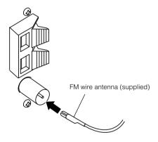
Fasten it up in the position until you have the best reception. If reception is poor, connect the outdoor antenna.
